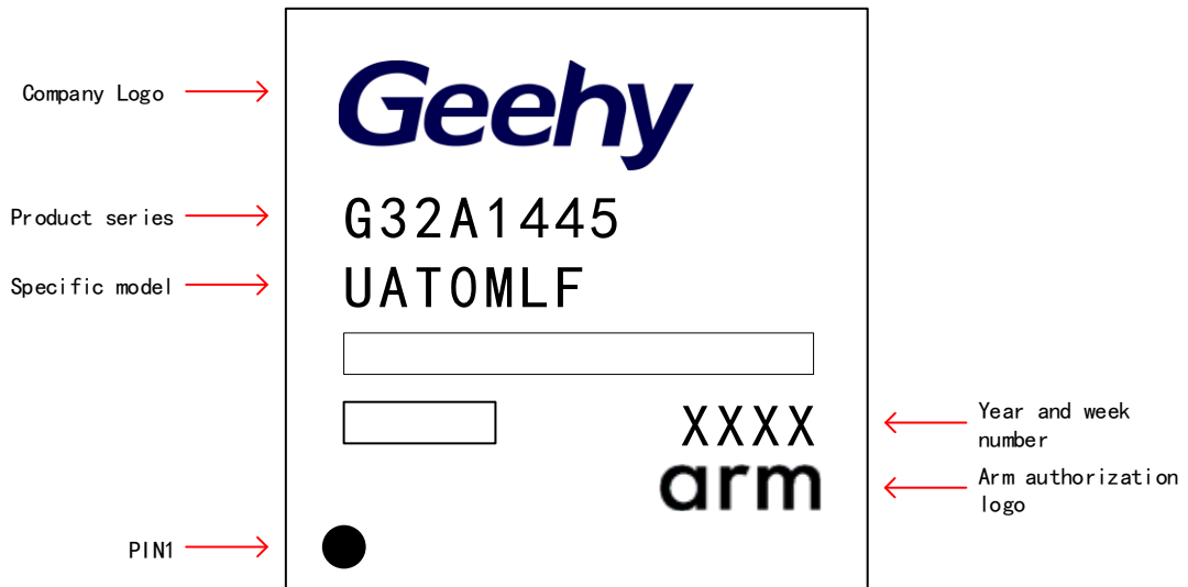
Figure 32 LQFP64 - 64 Pins, 7 x 7mm Diagram
